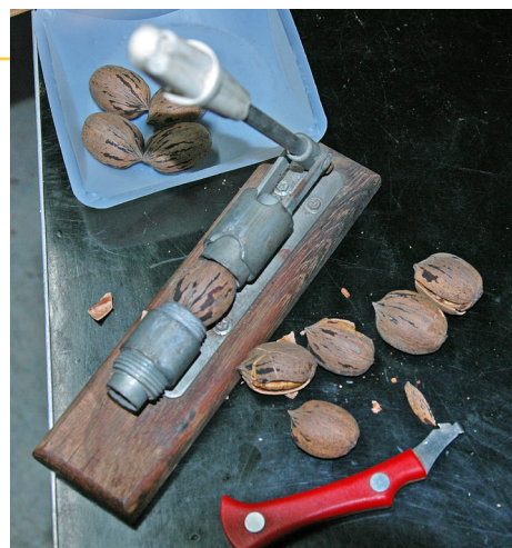
A lever-style tabletop sheller is designed for cracking pecans with minimal kernel breakage. After curing for 10 to 14 days, nuts shell more easily and produce cleaner halves. Use gentle pressure at both ends of the nut to avoid crushing the center.
