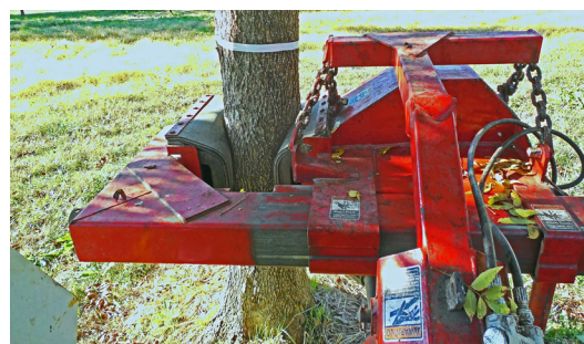
A hydraulic tree shaker clamps onto the trunk and vibrates a tree to dislodge mature pecans quickly. This method is common in commercial orchards but rarely used in home settings. If shaking by hand or with small equipment, wait until shuck split has begun to avoid damaging the tree or removing immature nuts. Photo by William Reid
