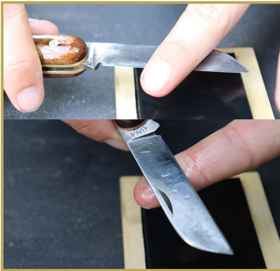
Figure 11. The top photo (A) is the safer method of testing for burrs based on the feel of the nonbeveled, flat side. The bottom photo (B) is a riskier way to test for burrs on the beveled side and is not recommended.
