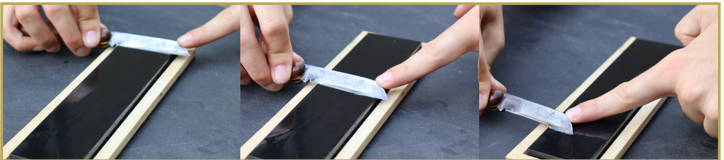
Figure 9. The process of how to pass a blade over a sharpening stone.
