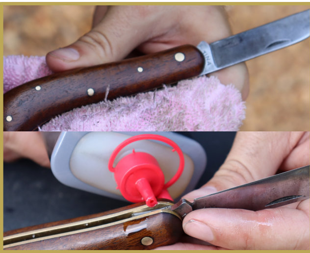
Figure 16. Oiling the wooden blade handle and pivot point on a grafting knife helps increase its lifespan.
