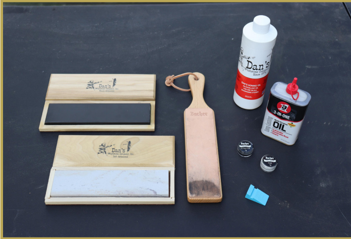
Figure 5. Tools for sharpening grafting knives include whetstones, leather strop, honing oil, polishing compound and angle guide.
