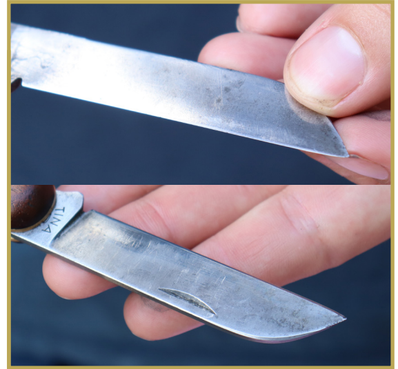
Figure 1. The top picture is the flat side of a grafting knife that has no bevel. The bottom picture shows the beveled side that is sharp.
