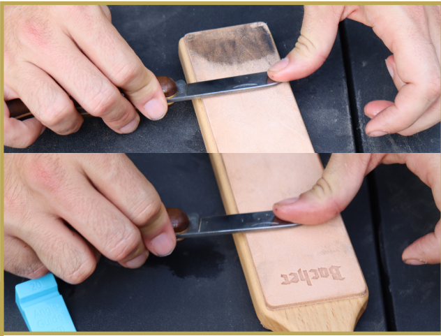
Figure 14. Stropping a knife over leather after sharpening can help remove burrs and lightly polish the knife.
