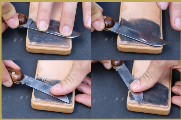
Figure 15. Polishing the knife on both sides after sharpening helps increase the knife's lifespan and contributes to a smoother, cleaner cut. The top pictures are polishing of the nonbeveled, flat side and the bottom pictures are polishing the beveled, sharp side.
