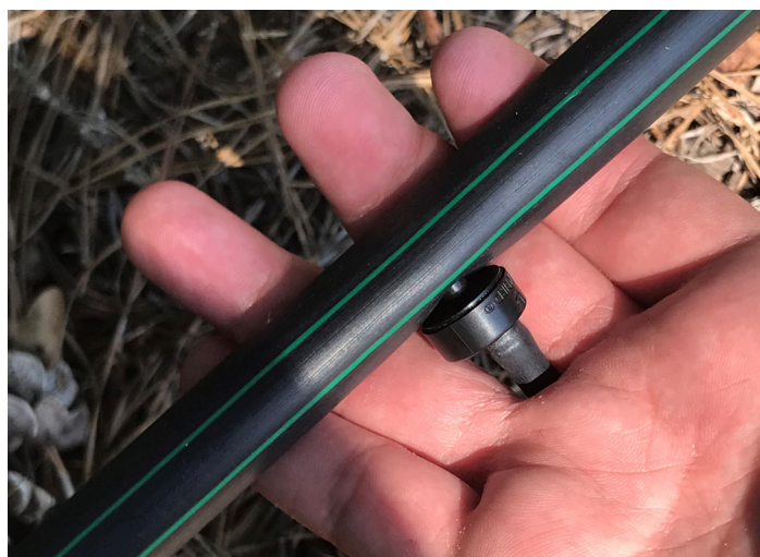
Drip line with an emitter installed.
