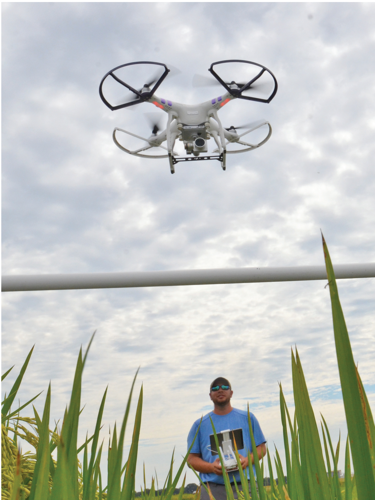
A drone flown by Brady Williams, LSU AgCenter research specialist, is used to pollinate hybrid rice at the H. Rouse Caffey Rice Research Station. The technique has been used on hybrid rice in China and is being tested at the station for its effectiveness.
