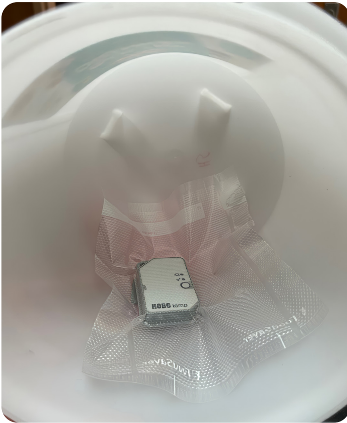
A temperature logger was placed inside each poultry drinker.
