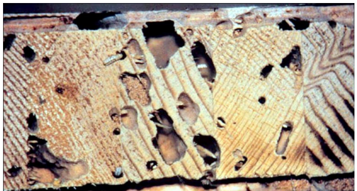
Wood damaged by Cryptotermes brevis (Rudolf H. Scheffrahn, University of Florida, Bugwood.org , Creative commons 3.0).
