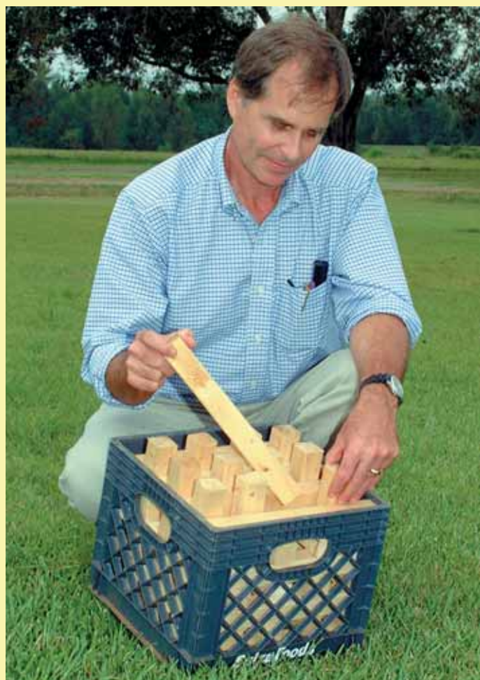
To test woods for termite resistance, Gregg Henderson uses milk crates which he fills with 44 sticks of wood 1 inch high by 1 inch wide by 12 inches long. He then buries the crates in an area known to be infested by Formosan subterranean termites.
