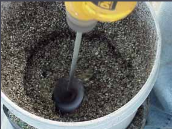
This procedure involves using a 24-inch auger mounted on a half-inch electrical drill to bore into the perlite in 5-gallon media bags without moving the bags.
