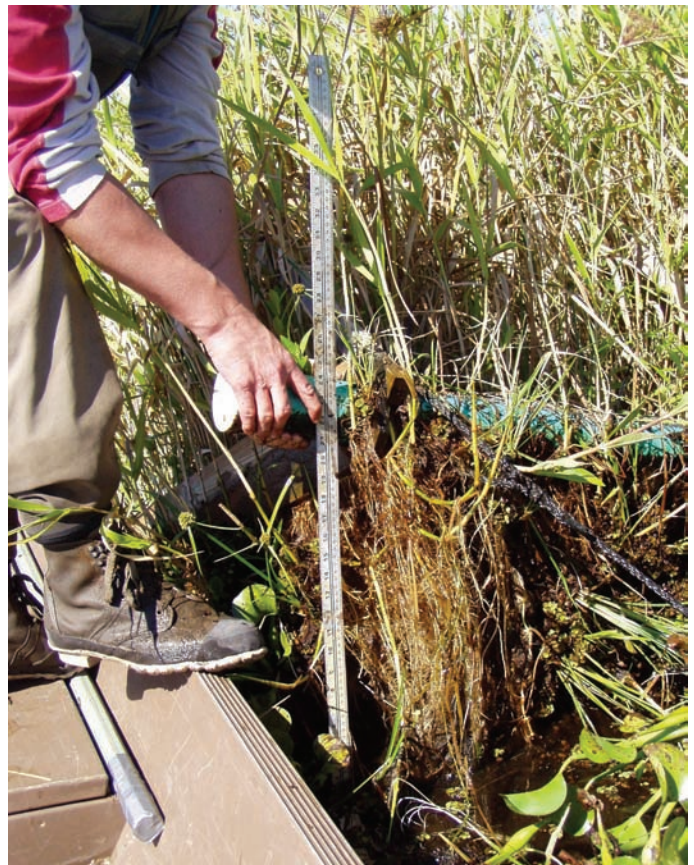
Figure 8. Measurement of root mat depth at the Mandalay marsh field site, October 2006.
