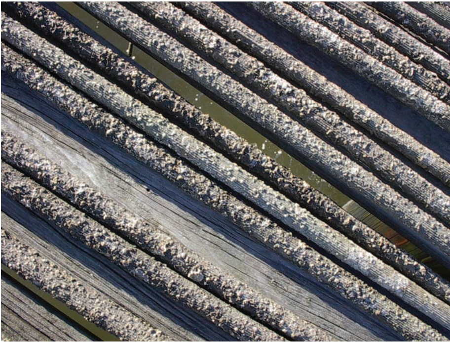
An early oysterbreak was made of "French tube," expanded and corrugated PVC pipe (above). The material provided habitat for oysters and barnacles as seen in the photo below. Other materials, however, have proved to provide a better place for oysters to live.
