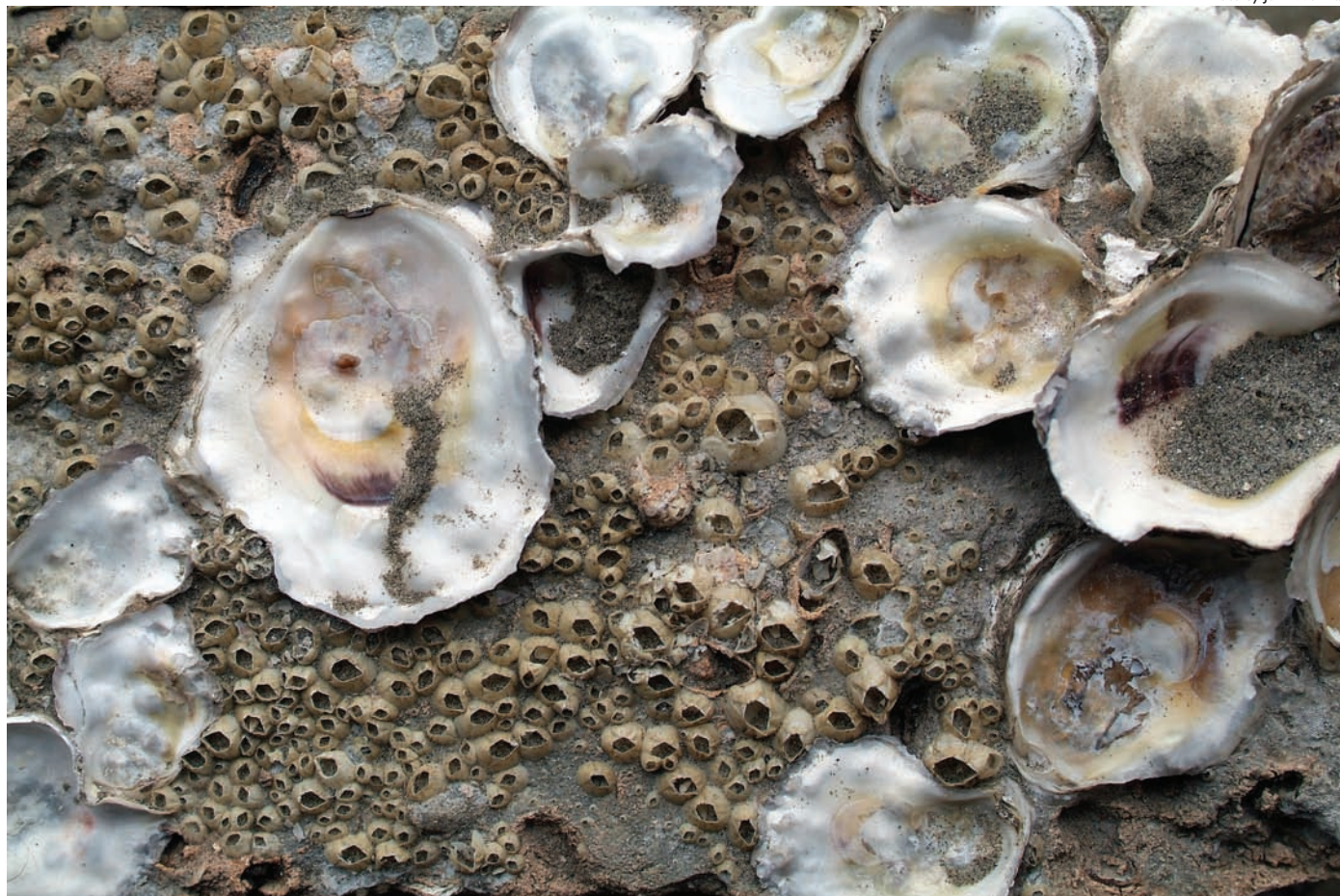
This close-up of a concrete and agricultural byproduct material shows oysters – the largest here about 2 inches long – thrive on this material. This particular substrate had been in the Gulf of Mexico off Grand Isle for about three months when it was removed for the photograph.
