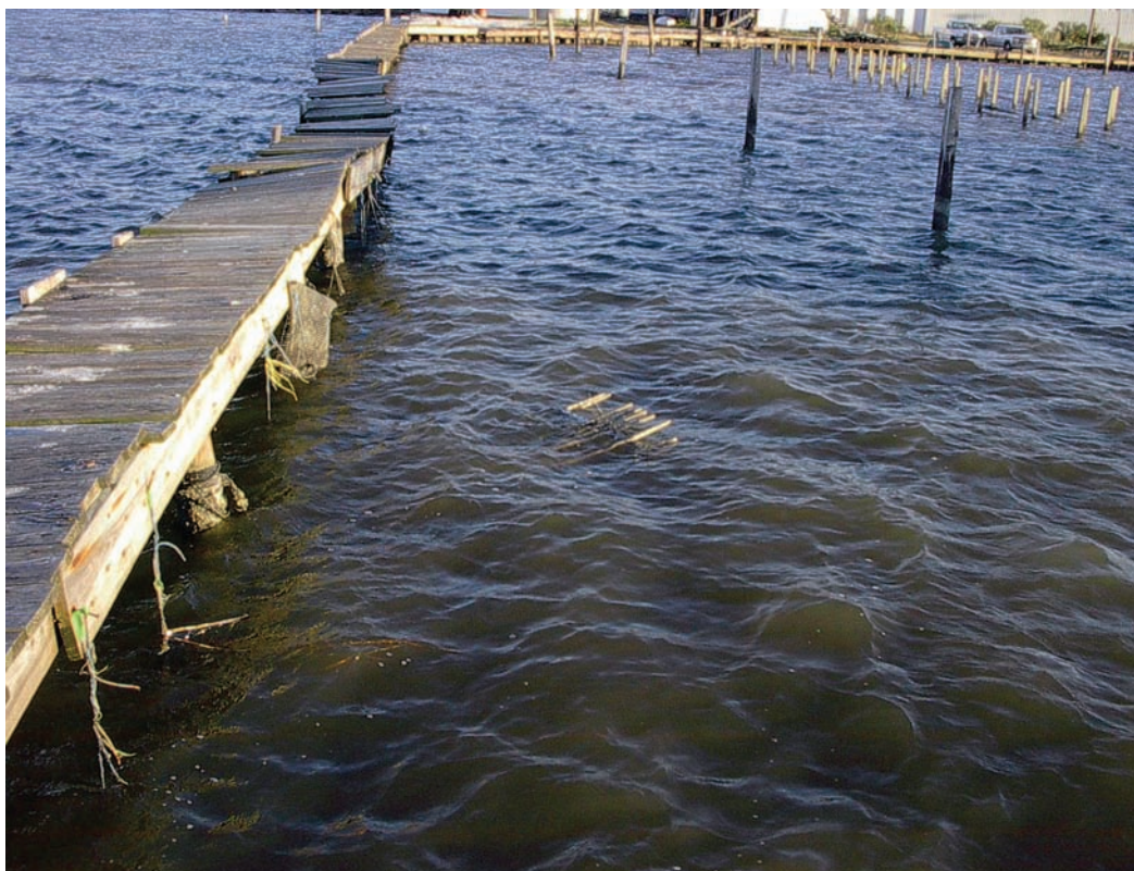
A section of a full-size oysterbreak (above) was built and deployed at the LSU oyster hatchery facility at Grand Isle in 2004. The structure is made of "French tube" – expanded and corrugated PVC. The 5-foot-high structure was placed in the water (below) to evaluate its ability as a home for oysters. The area behind the oysterbreak contains a "long-line" system that allows oyster producers to pull up and lower down materials on which oysters live. The area where the oysterbreak was tested allows the structure to be slightly submerged at low tide.
