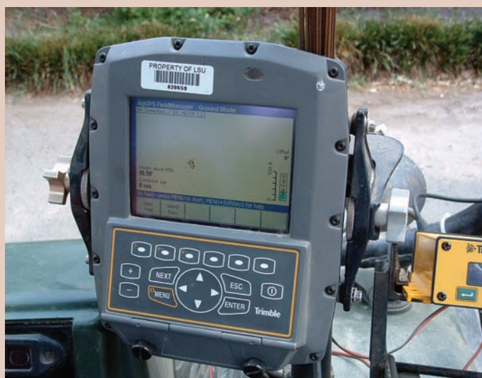
Researchers use this GPS device to pinpoint field locations to match maps developed using electrical conductivity, which can be used to differentiate soil types.
