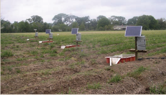
Edge-of-field runoff collections were sampled for contaminants using automatic water samplers, and runoff volume was measured by flow meters.
