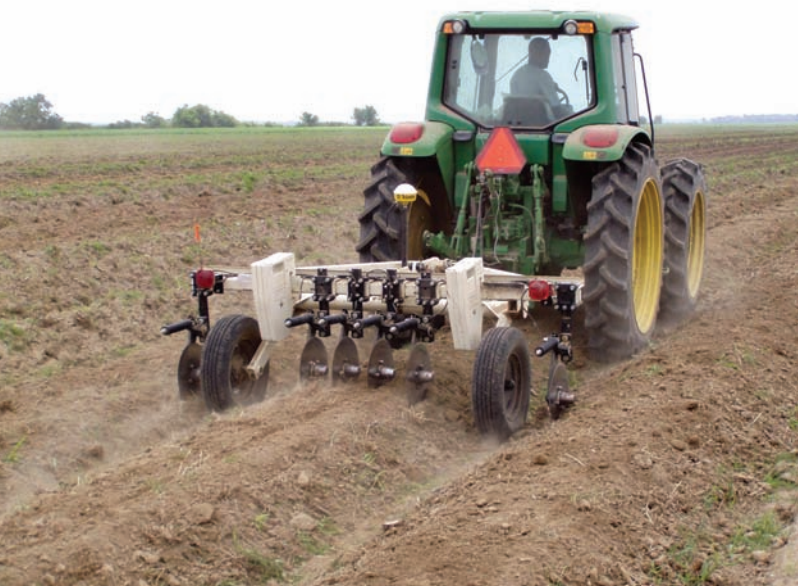
Veris cart measuring electrical conductivity at two soil depths (zero-to-1-foot and zero-to-3-feet) and soil grid sampling pattern at Gralyn Plantation in Iberia Parish showing Jeanerette (Ja) and Patoutville (Pa) silt loam soils.
