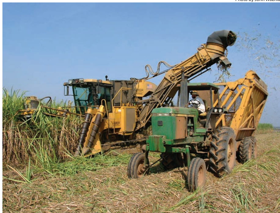
A chopper harvester is capable of lifting lodged (fallen over) cane and cutting it into sections called billets.
