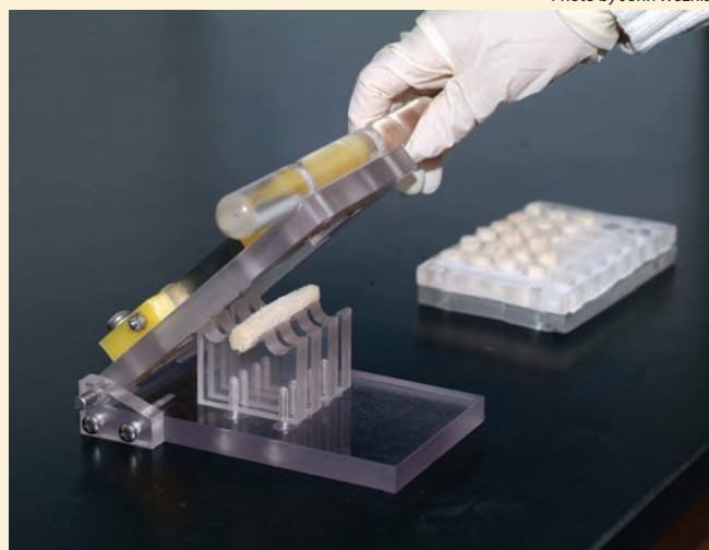
Testing for ratoon stunting disease involves removing cores from stalks and cutting them into pieces. The LSU AgCenter operates the Sugarcane Disease Detection Laboratory to aid Louisiana's sugarcane industry.
