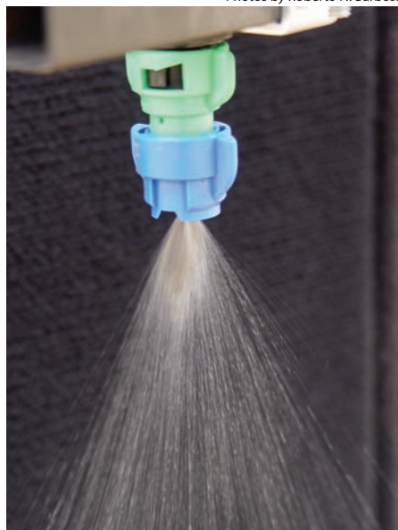
Figure 1. Hydraulic nozzles with single jet technology distribute all liquid through a single orifice. They can form spray angles of 80 or 110 degrees.
