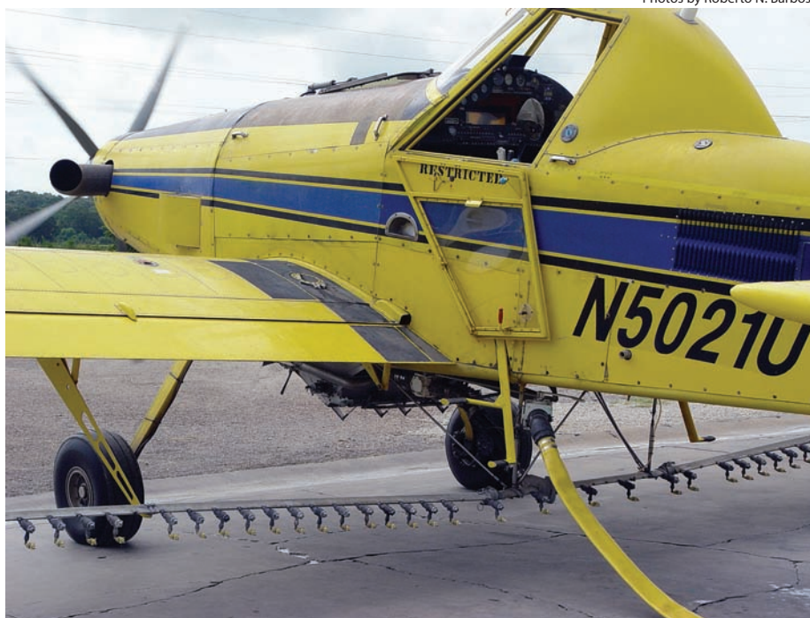
During spraying season, sprayers should be kept clean and nozzles should be checked, cleaned and replaced when worn.
