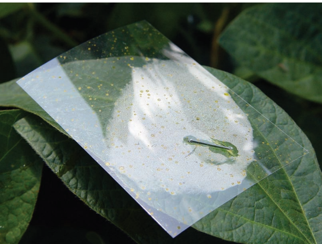
Small cards, measuring 2 by 3 inches, were distributed throughout the plant. Deposits of tartrazine in the cards were detected in the laboratory using colorimetry.
