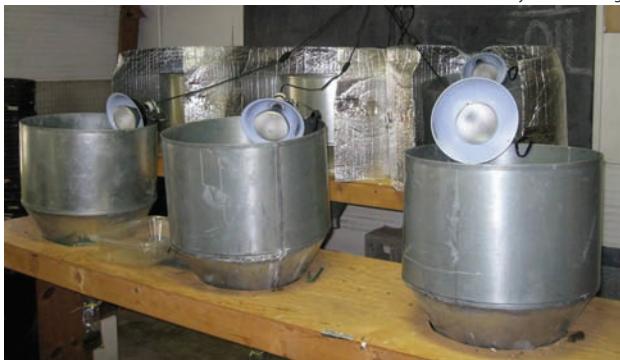
Figure 3. Weevil density estimates are obtained by processing a known weight of salvinia on the Berlese Funnel, which is a separation and extraction device that relies on positive geotaxis in response to the desiccation of the plant material on a screen beneath a 125-watt heat lamp, which forces the weevils down the funnel into a collection bag with a few salvinia plants.
