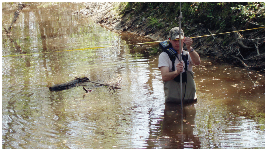
Measuring stream flow in Flat Creek. Photo by Y. Jun Xu
