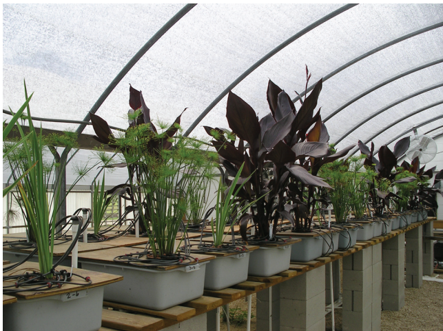
Ornamental canna Australia and dwarf papyrus being evaluated for the ability to remove excess nutrients from stormwater in a nutrient-recirculating research system. Photo by Yan Chen
