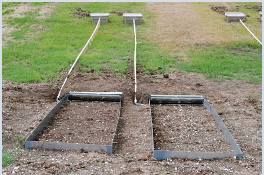
Trays used for surface runoff collection. Photo by Robert Burwell Jr.
