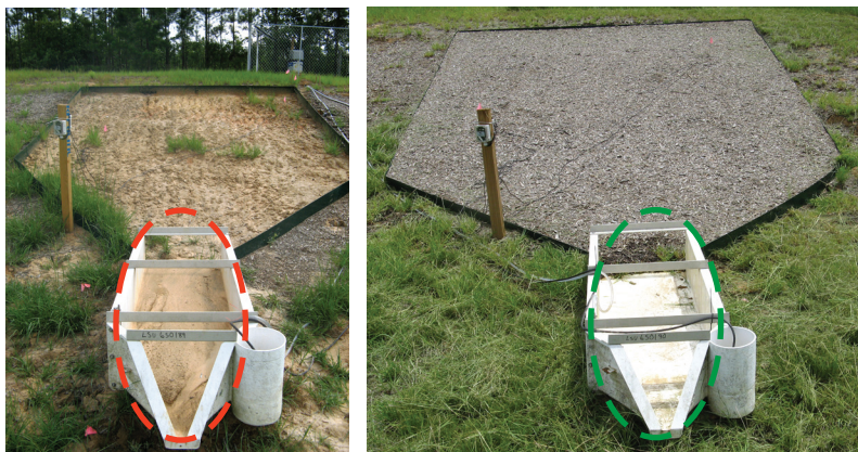
Sediment generated by control plots with no compost/mulch (left) and 4 inches of compost/mulch application (right) in test plots along I-49 in Rapides Parish. Photo by David C. Weindorf
