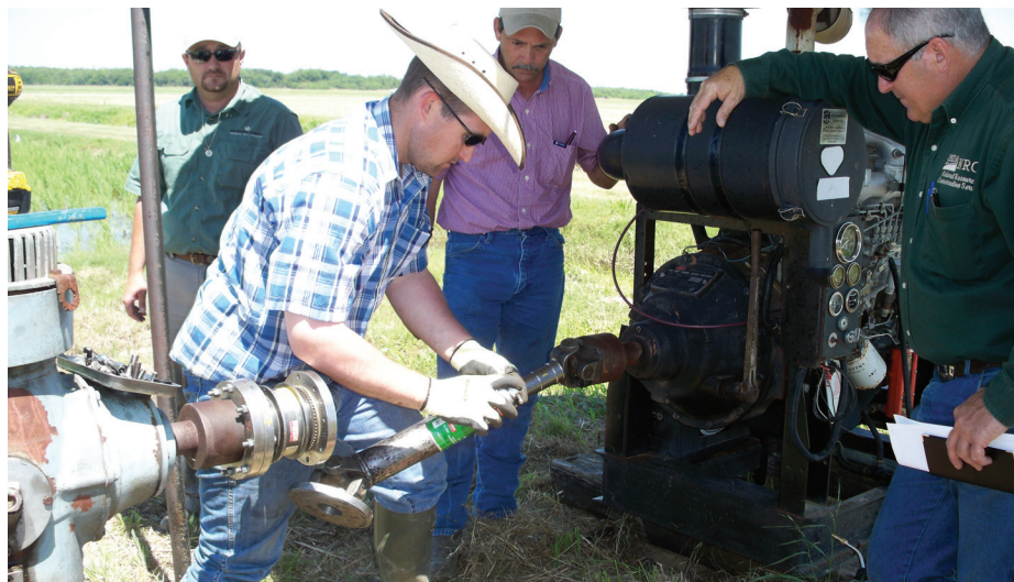
Nich Kenny, of Texas Agri-Life Extension, demonstrates how to install a torque cell on a diesel-powered irrigation pump.
