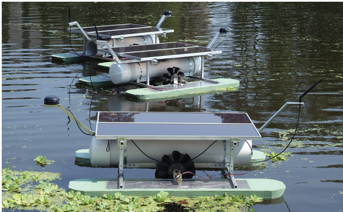
Multiple vehicles can cooperate to perform aquatic tasks. The round black devices floating along the side have GPS and provide location and speed, while antennas on the opposite end can send and receive signals from the other boats. Photo by John Wozniak
