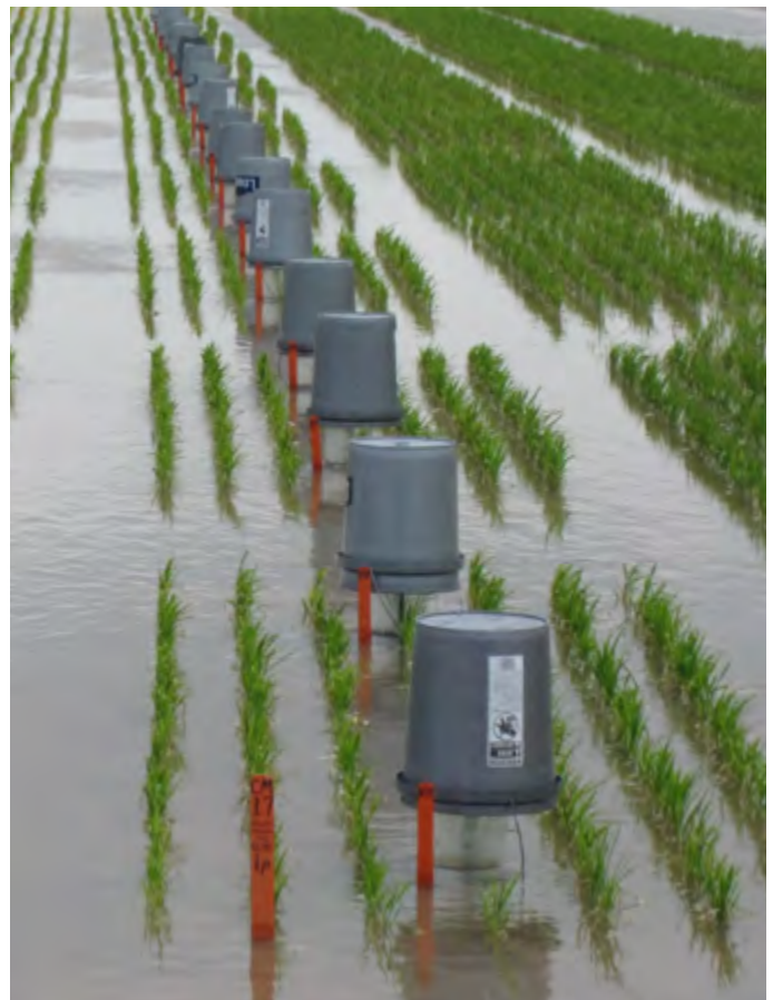
Semi-open volatilization chambers are used to capture volatilized ammonia gas from nitrogen fertilizers. Ammonia is captured for 15 days after nitrogen fertilizers are applied. The permanent flood is established on day 10. Photo by James Leonards
