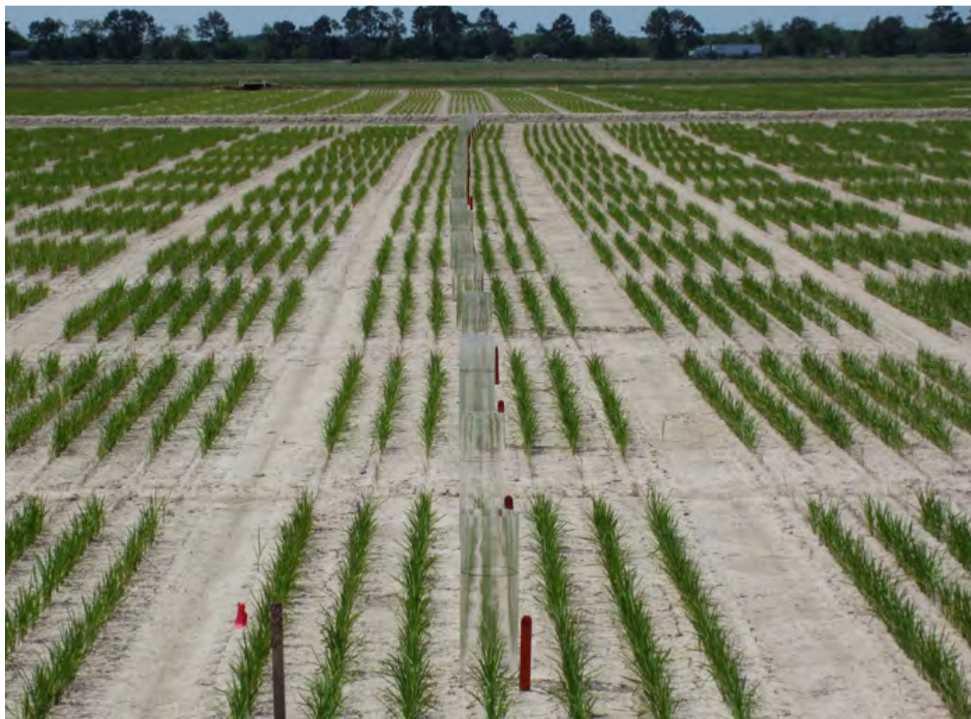
Photo 2. Plexiglas tube which is used as the housing of the semi-open volatilization chambers used in nitrogen volatilization trials. Photo by James Leonards
