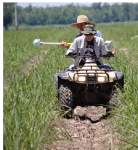
Payton Dupree, in front, and Brandon White, graduate students, collect sugarcane canopy reflectance readings using GreenSeeker sensor from a nitrogen field demonstration plot in Donaldsonville. Photo by Brenda S. Tubaña
