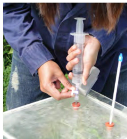
Gas samples are collected from an enclosed chamber with potted rice plants in a study on methane emission in rice production. Photo by Brenda S. Tubaña
