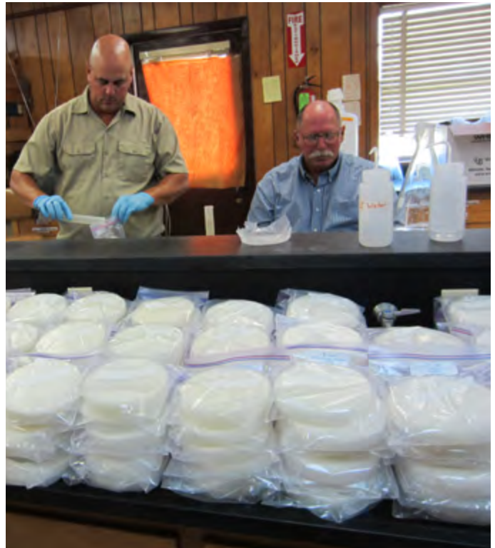
Research associates James Leonards (left) and Ronald Regan (right) shown extracting acid-trapped ammonium from sponges used to capture ammonia gas volatilized from surface-applied nitrogen fertilizers. Photo by Dustin L. Harrell
