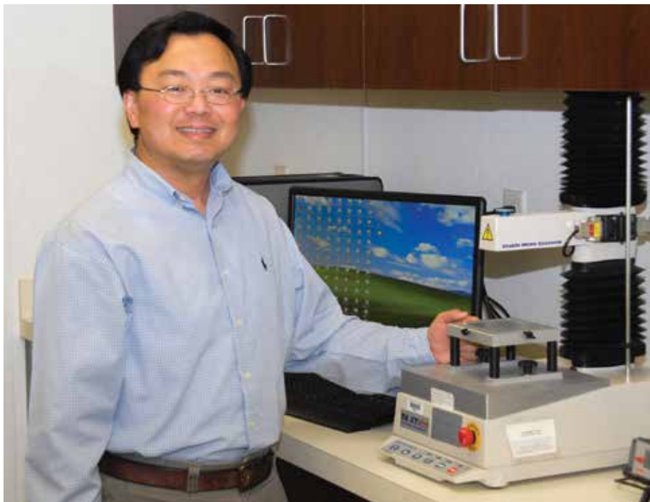
LSU AgCenter researcher Witoon Prinyawiwatkul explains a texture analyzer that's used to measure the hardness and springiness of food samples. The equipment is in the new Animal and Food Sciences Laboratories Building on the Baton Rouge campus. Photo by Rick Bogren
