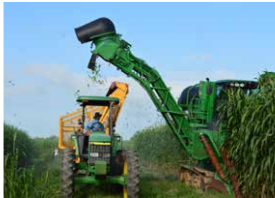
Energycane grown at the LSU AgCenter Sugar Research Station in St. Gabriel is harvested and transported with machinery used for commercial sugarcane. This existing machinery can be used without modification for both energycane and sweet sorghum. Energycane is a high-fiber, low-sugar-content sugarcane grown for use as a feedstock for biofuels. Photo by A. Denise Attaway
