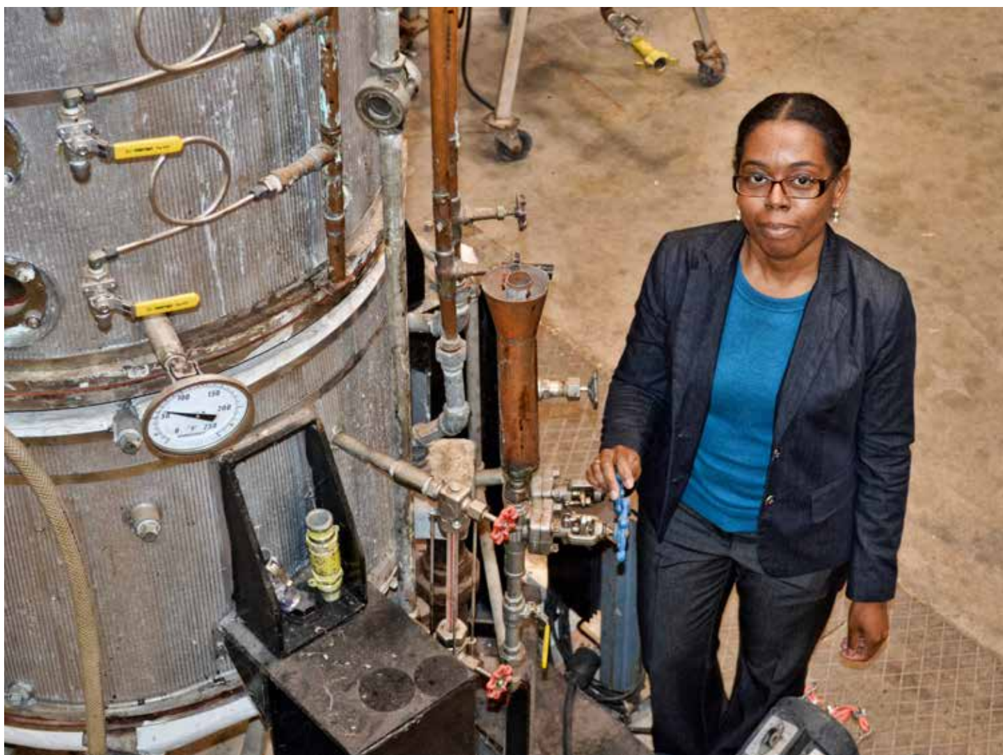
Daira Aragon, an assistant professor at the LSU AgCenter Audubon Sugar Institute, stands next to an evaporator where juice extracted from energycane and sweet sorghum could be processed to make biofuels. Photo by A. Denise Attaway
