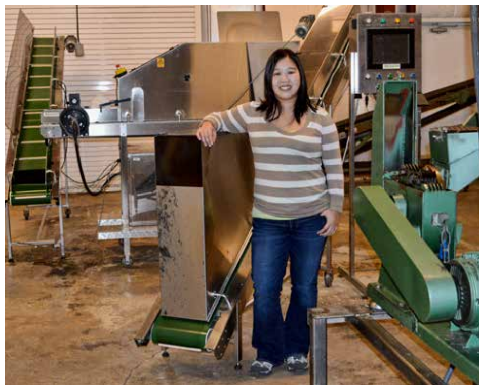
Shyue Lu is pictured with the Spectracane near infrared spectroscopy system at the Sugar Research Station in St. Gabriel. Whole stalks of energycane and sweet sorghum are fed directly into the Spectracane for analysis. Photo by Denise Attaway
