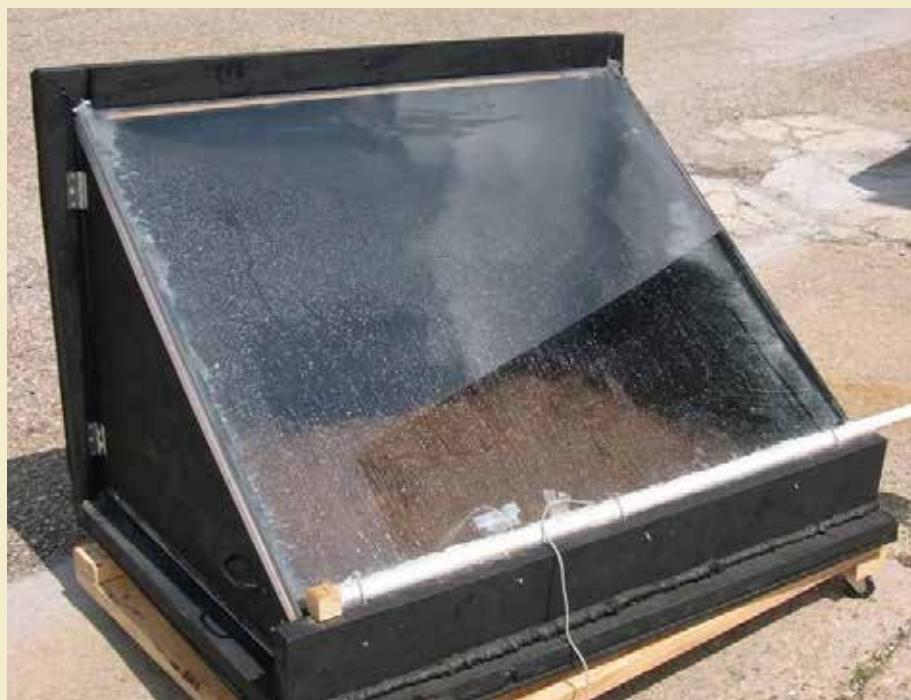
Figure 1. Incident solar radiation heats the solar still to very high temperatures (about 210 degrees F during midday). In the regular non-convection mode (with no air blower), water evaporated from the wet waste condenses on the cooler glass surface and runs to the bottom of a special channel to be drained out. In the convection drying mode (with air blower), water is carried away with incoming fresh air. This concept was validated in the Department of Biological and Agricultural Engineering using separated dairy manure in smaller, custom-built solar stills.
