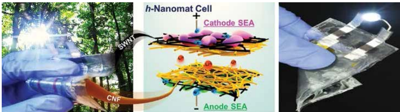
Figure 4. Flexible rechargeable Li-Ion battery based on nanocellulose technology. (dx.doi.org/10.1021/nl5024029 | Nano Lett. 2014, 14, 5677–5686)
