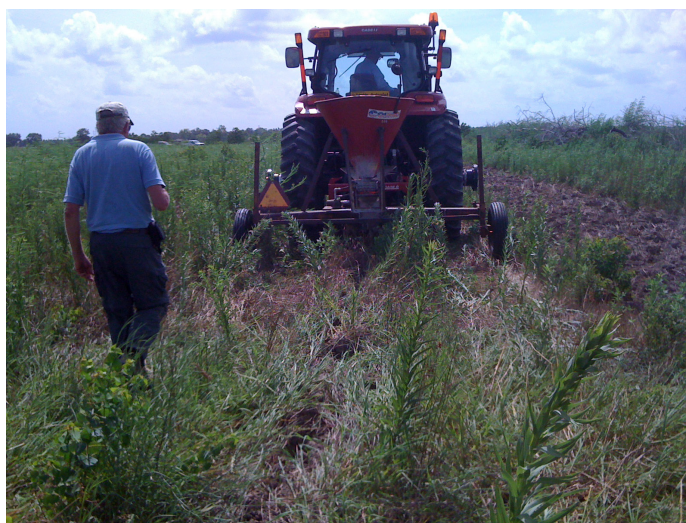
Figure 2. Fertilizer dispenser mounted to a subsoil plow used to prepare a field in southeastern Texas for eucalyptus planting. Photo by Michael Blazier.
