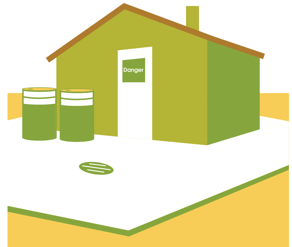
Figure 5.3. Maintain a well-designed, secure pesticide storage facility with highly visible warning signs. Keep it well-ventilated and located where water damage is not likely to occur.
