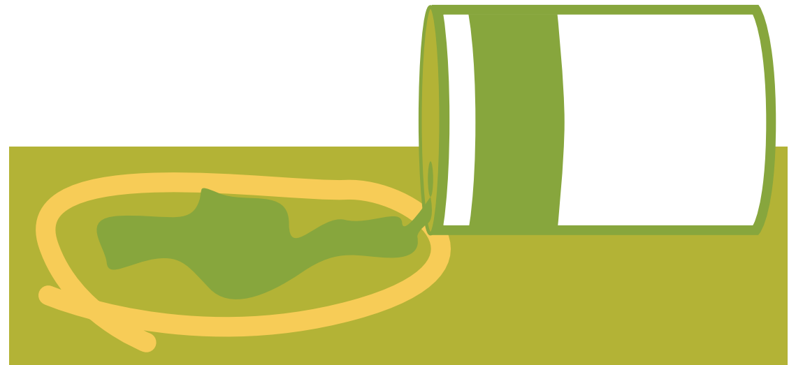
Figure 4.5. Take action to prevent spills from spreading. In this case, an absorbent spill tube is used to contain the spill.
