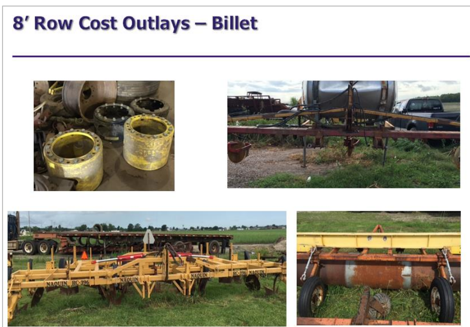
Figure 2. Billet equipment modification performed by project cooperators. Clockwise: folding boom sprayer modification, roller implement, row cultivation implement, and tractor wheel hub modification.
