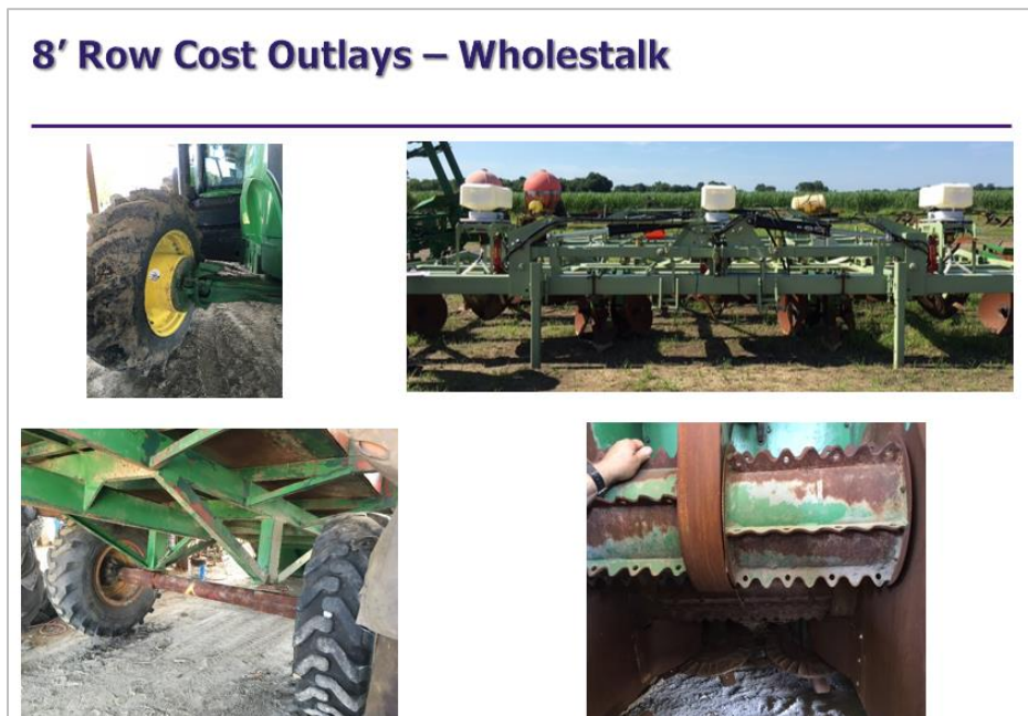
Figure 1. Whole stalk equipment modification performed by project cooperators. Clockwise: row cultivation implement, harvester modification to chopper, axel modification for planting wagon, and tractor wheel hub modification.
