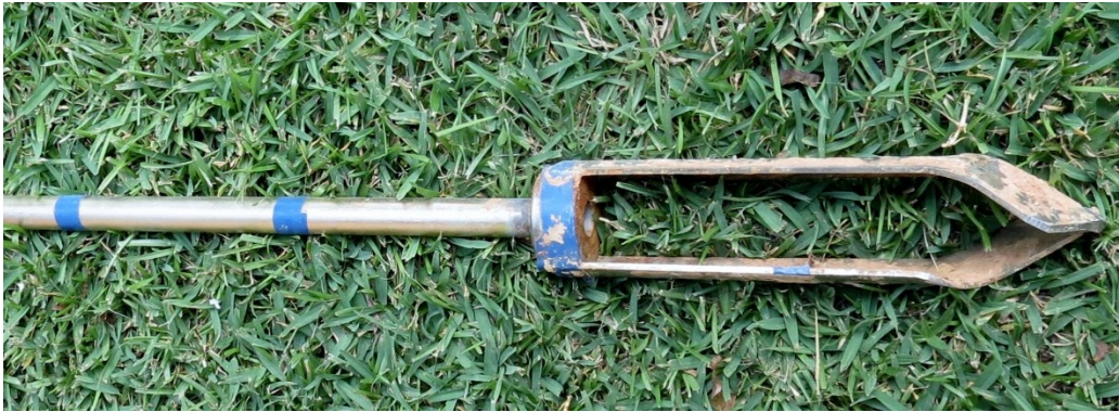
Figure 4. Electrical tape placed at 6in increments on clay auger.
