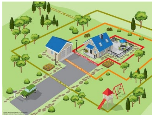
Figure 3. Diagram of 'Defensible Space' zones for a suburban home setting. Reproduced with permission from the National Fire Protection Association, copyright © 2019, NFPA, Quincy, MA. All rights reserved.
