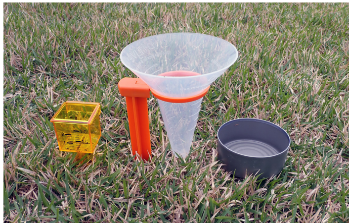
Figure 1. Collect the equipment needed for the audit, including a rain gauge or graduated cylinder, 12 or more catch cups and your phone for a timer.
