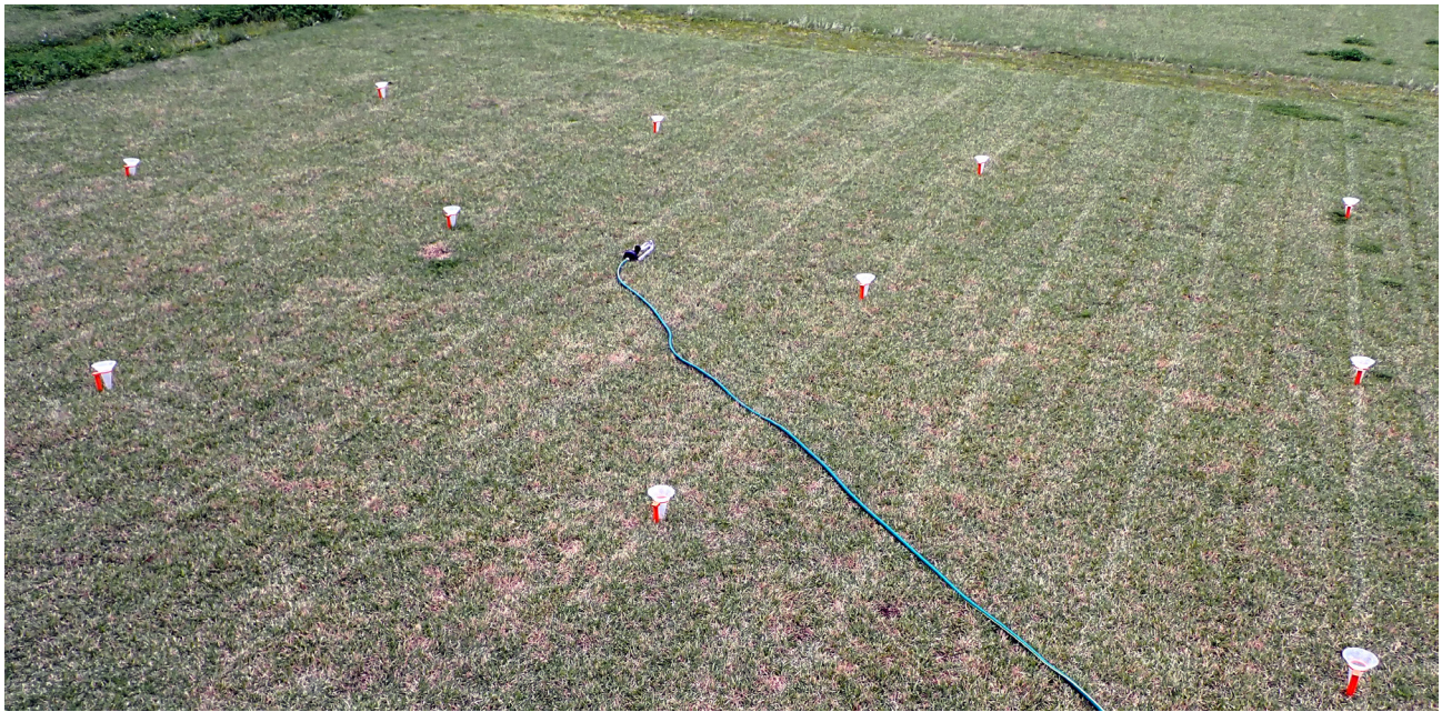
Figure 2. Evenly space catch cans in a grid representing the area being irrigated by a specific sprinkler or irrigation zone. The more cans used, the more accurate the results will be.
