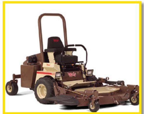
Figure 9. ZTR mower with front-mount deck. Homeowner machines are generally mid-mount. Each configuration has advantages and disadvantages, and each has proponents. Mid-mount decks are much more popular than front-mount decks.
