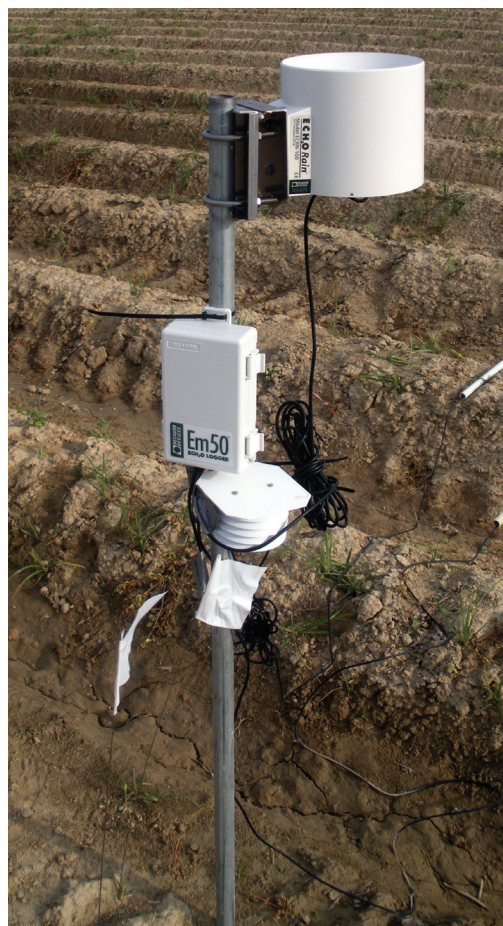
Photo 4: Weather station used at each field site to measure agroclimatic variables. Photo by Theresa Arnold
