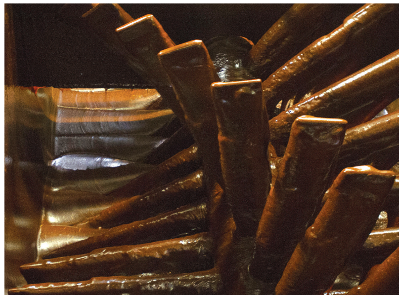
Massecuite flowing through the crystallizers. Massecuite is a mixture of molasses and sugar, just before their separation. Photo by Olivia McClure
