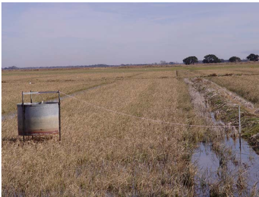
Figure 10. A drop sampler, set and ready to trip with a slight tug on the rope from the levee. Crawfish are retrieved by pumping out the water from the caisson while the cylinder walls are in contact with the mud bottom, exposing any crawfish trapped within. Rice Research Station, Crowley, LA. 2007.
