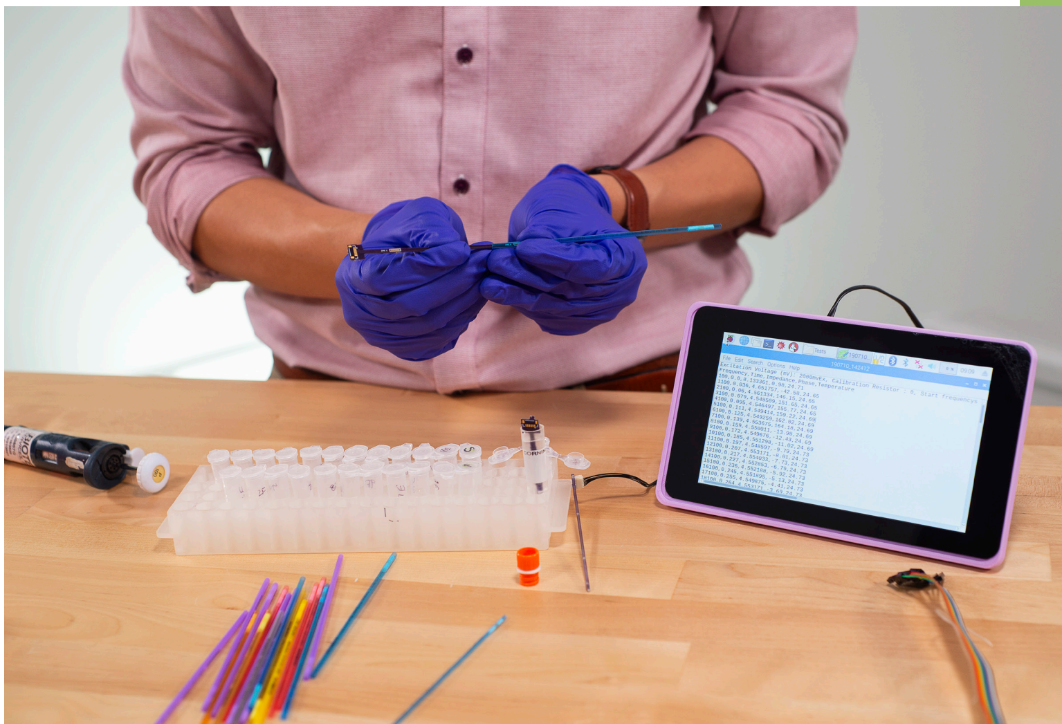
Researchers from the Aquatic Germplasm and Genetic Resources Center developed customized sensors to monitor the changes in temperature and electrical properties of sperm samples during cryopreservation. The figure shows sensors fabricated by use of printed circuit board being inserted into a standard cryopreservation straw and vial. Photo by Olivia McClure
