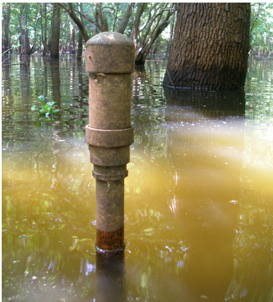
A water monitoring station emerges from receding floodwaters. Extensive instrumentation will make the Forested Wetlands Observatory an attractive site for a range of scientific objectives. Photo by Richard Keim
