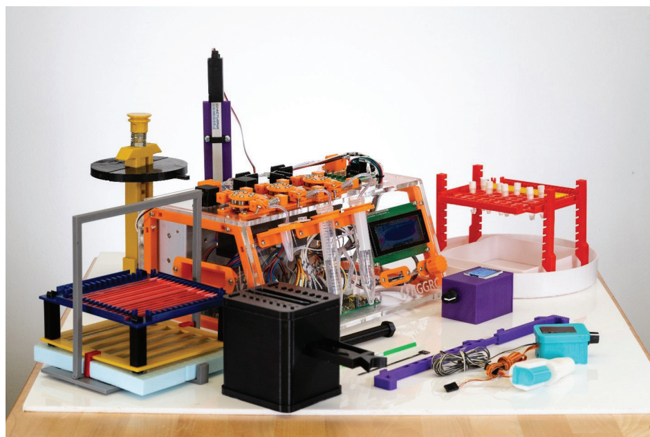
Figure 2: Innovative technologies are developed at the AGGRC in the form of open hardware that can be shared as computer files with user communities to support use of germplasm repositories. These devices address steps in sample processing, freezing and thawing, and are custom designed for fabrication by use of consumer-level 3D printers, electronics and microcontrollers.
