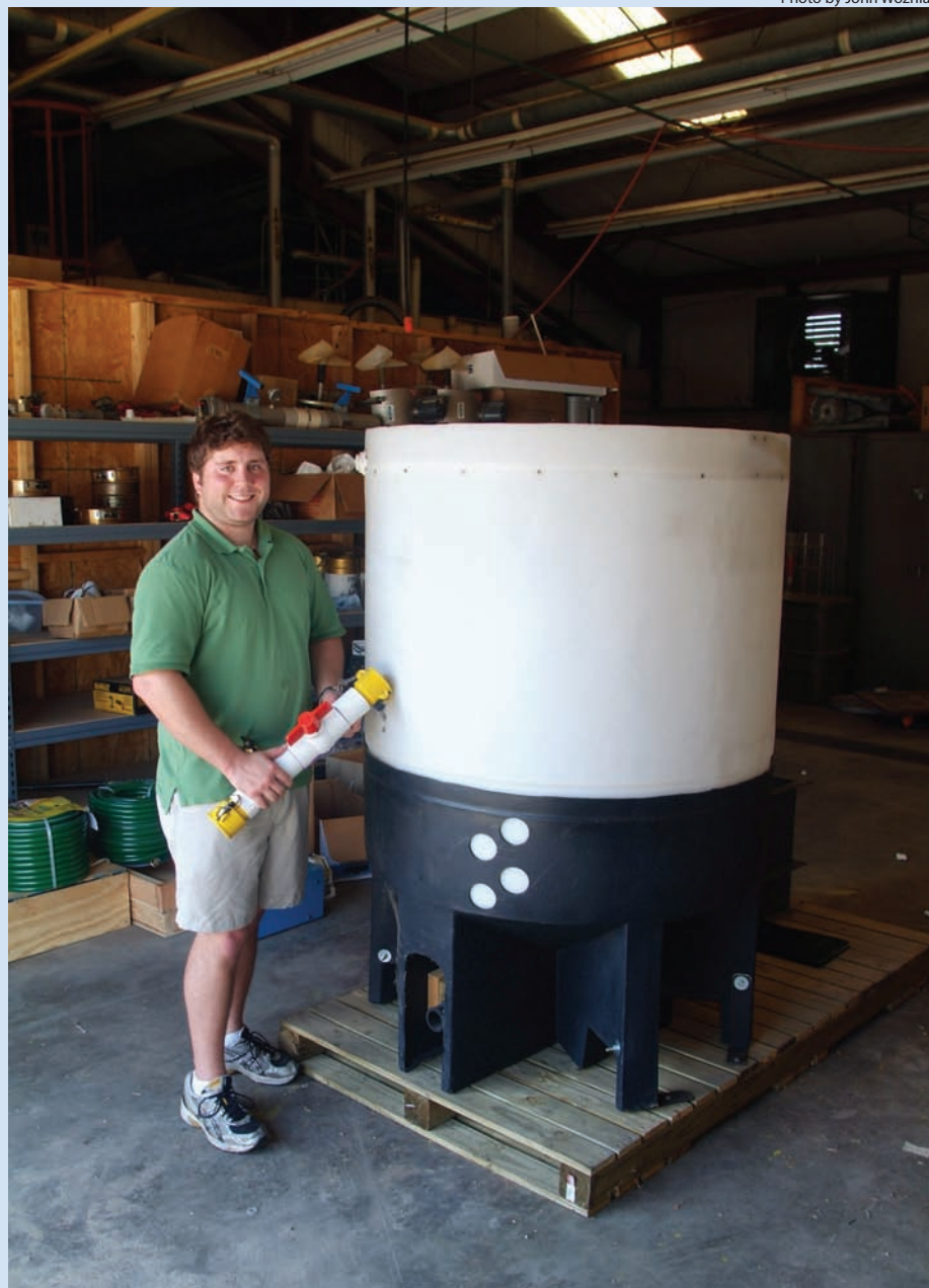
Troy Davis with a portion of the lime-precipitation unit under construction in the Department of Biological & Agricultural Engineering.
