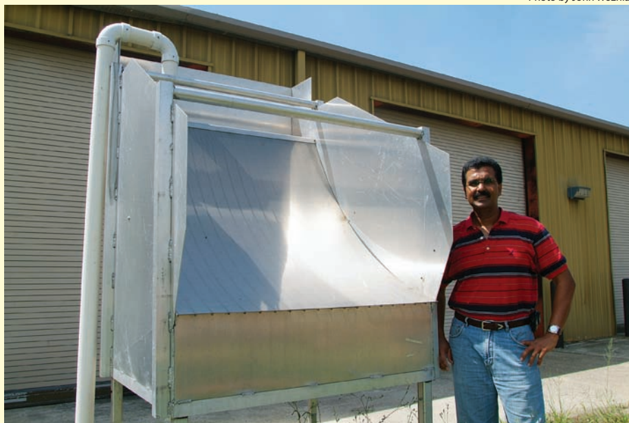
Figure 2. Self-cleaning dairy manure and sand separator developed at LSU AgCenter. This screen next to Chandra Theegala, separates organic matter and sand into separate piles.
