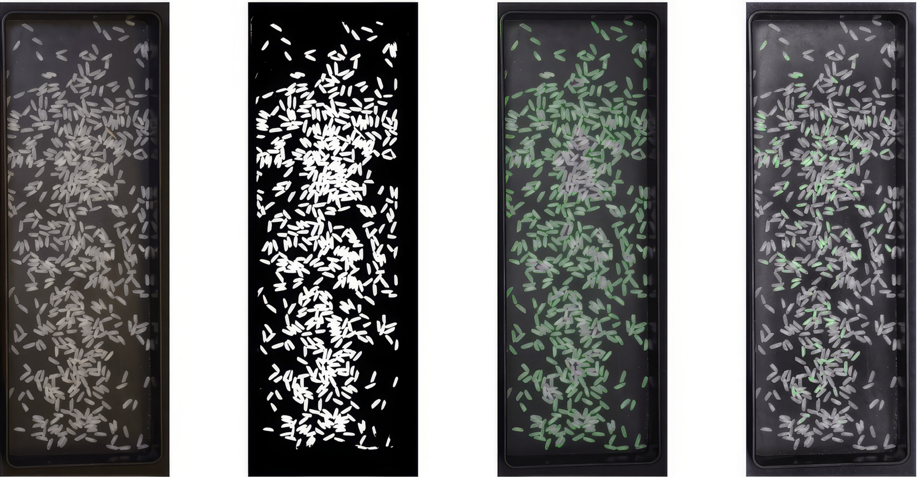
Researchers analyzed the images of rice produced from the LSU AgCenter's breeding program to evaluate grain characteristics like chalkiness, milling and grain length at the H. Rouse Caffey Rice Research Station. Photo by Jardel da Silva Souza
