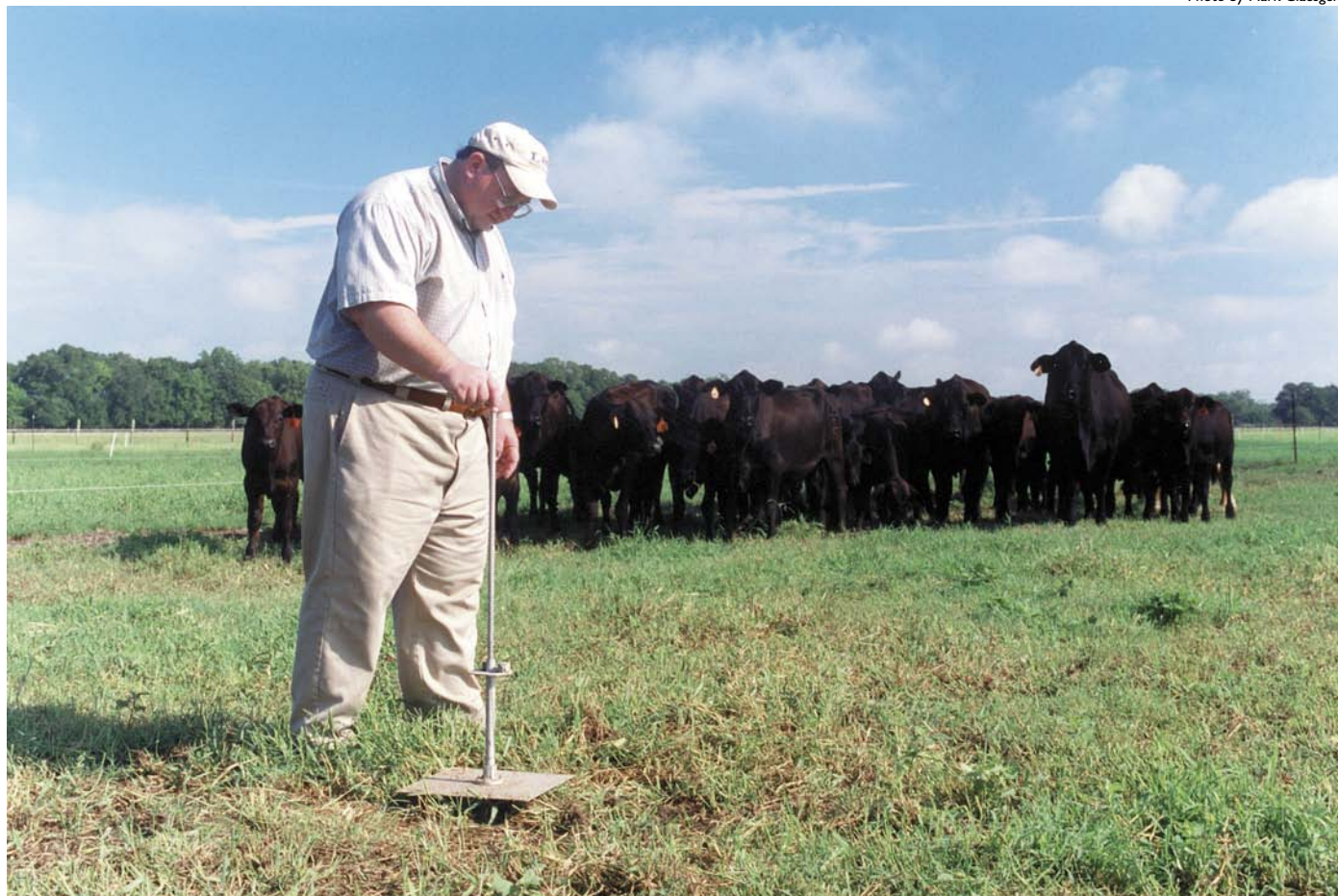
Wayne Wyatt uses a rising plate meter to estimate the amount of forage available for grazing on a pasture. This is part of a research project at the LSU AgCenter's Iberia Research Station near Jeanerette to examine the net returns of grazing systems that either rotate grazing cattle among several smaller pastures or allow them to continuously graze on one larger pasture. Shown is a group of about 18 cow-calf pairs that rotationally graze eight 2-acre paddocks throughout the year.
