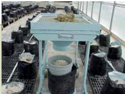
Figure 1. A movable hopper with a wire mesh screen is used for sifting the perlite.
