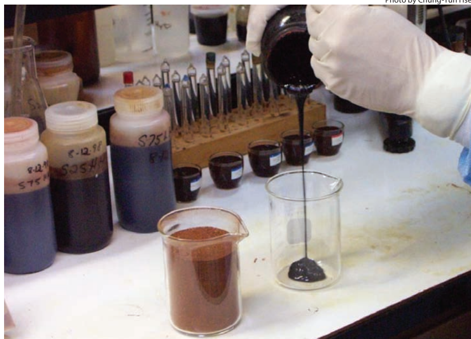
Figure 1. Wood particles (left) and liquefied wood (right) being poured into a beaker.
