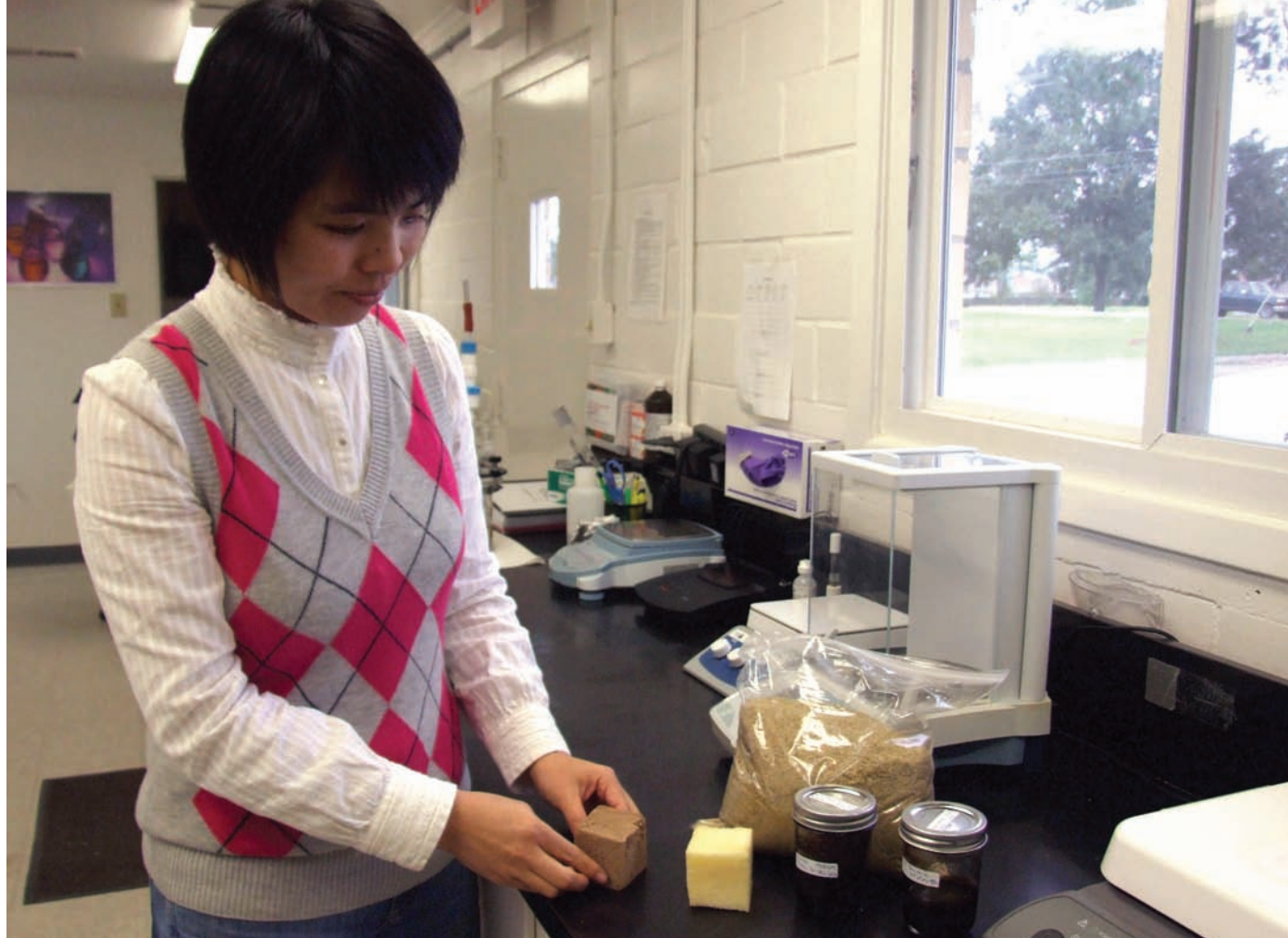
Hui Pan, assistant professor at the Calhoun Research Station, holds samples of polyurethane foam made from liquefied wood. The foam is free of heavy metals and safe for the environment.
