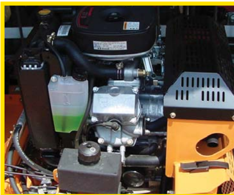
Figure 5. Water-cooled engine on commercial ZTR mower.
