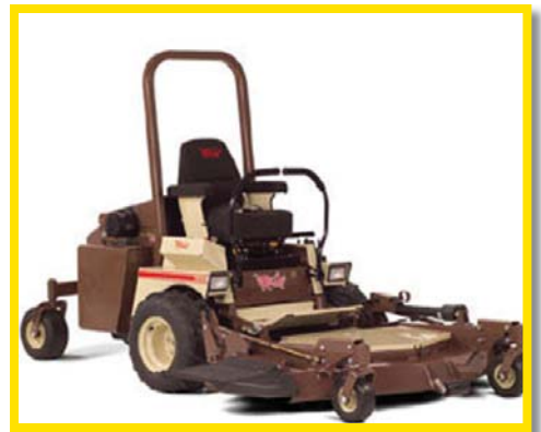
Figure 9. ZTR mower with front-mount deck. Homeowner machines are generally mid-mount. Each configuration has advantages and disadvantages, and each has proponents. Mid-mount decks are much more popular than front-mount decks.
