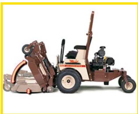
Figure 13. Tilt-up deck on front-mount ZTR mower.
