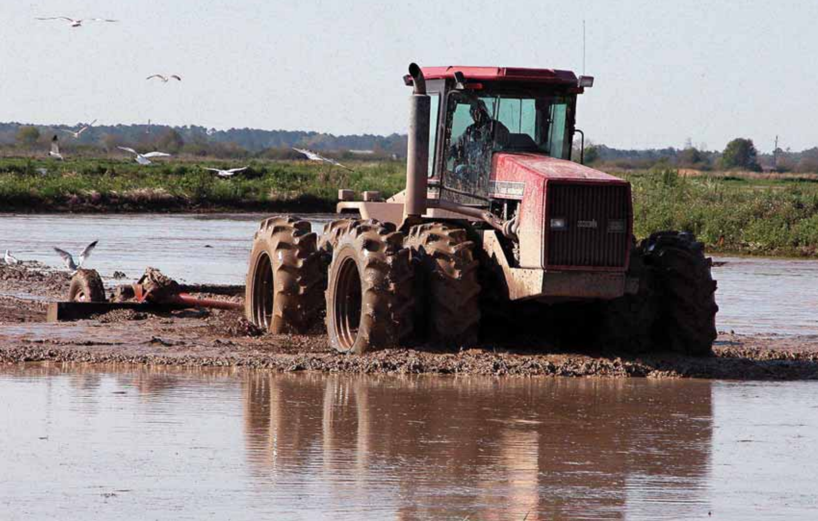
A rice farmer between Eunice and Crowley water-levels his field before planting. This is the traditional method. The alternative is laser-leveling, which is more accurate but more expensive.
