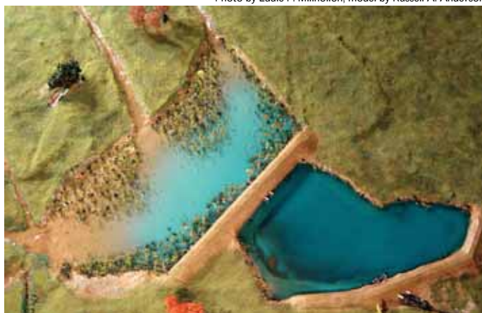
This is a photo of a model of the constructed wetland showing the shallow and deep cells and drainage ditches that carry runoff over the 400 acres.
