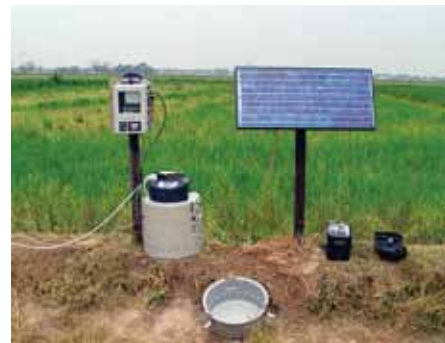
The equipment includes an automated runoff collection sampler, bubble flow meter and solar panel and battery for equipment power.
