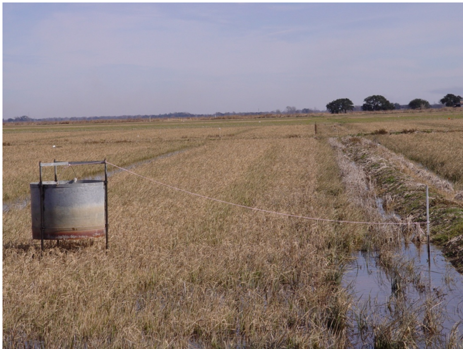
Figure 10. A drop sampler, set and ready to trip with a slight tug on the rope from the levee. Crawfish are retrieved by pumping out the water from the caisson while the cylinder walls are in contact with the mud bottom, exposing any crawfish trapped within. Rice Research Station, Crowley, LA. 2008.
