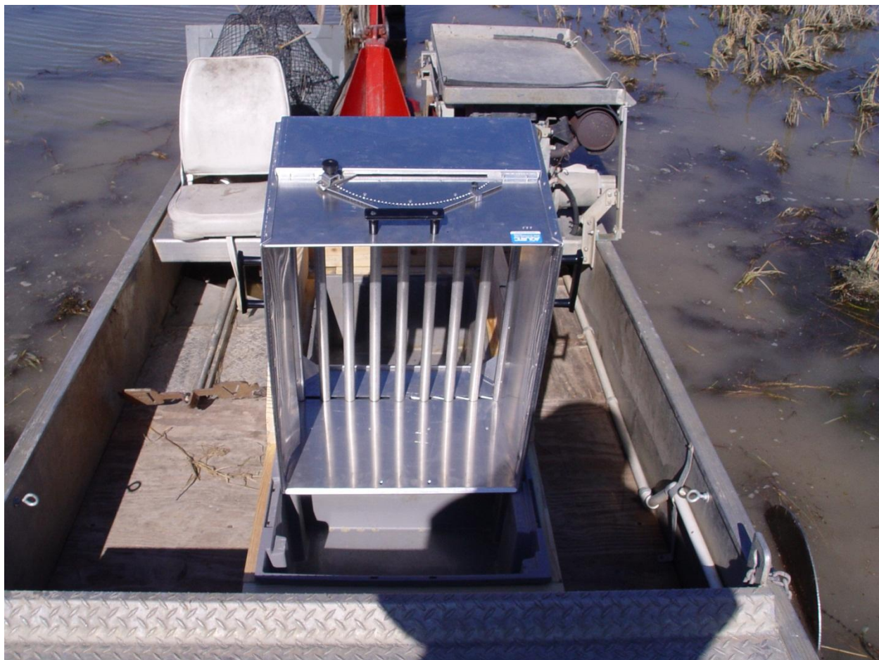
Figure 1. Size grading of crawfish was accomplished in the boat at harvest with a variable fish grader. Grader was adjustable for different size categories.
