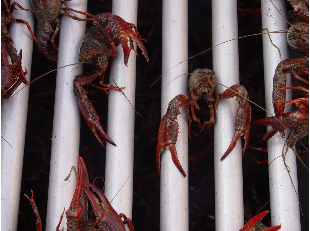
Figure 3. Size grading in crawfish is accomplished according to width of the carapace.
