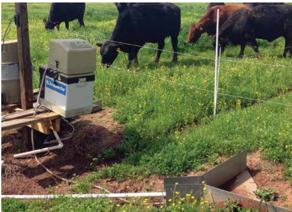
The water samplers use suction lines and water sensors to initiate sampling after rainfall events begin. A computer program inside the sampler is used to determine the amount of sample collected, how often, etc. Samples are collected and analyzed for solids, phosphates, total phosphorus, nitrates and potassium. Photo by Jeff Gurie
