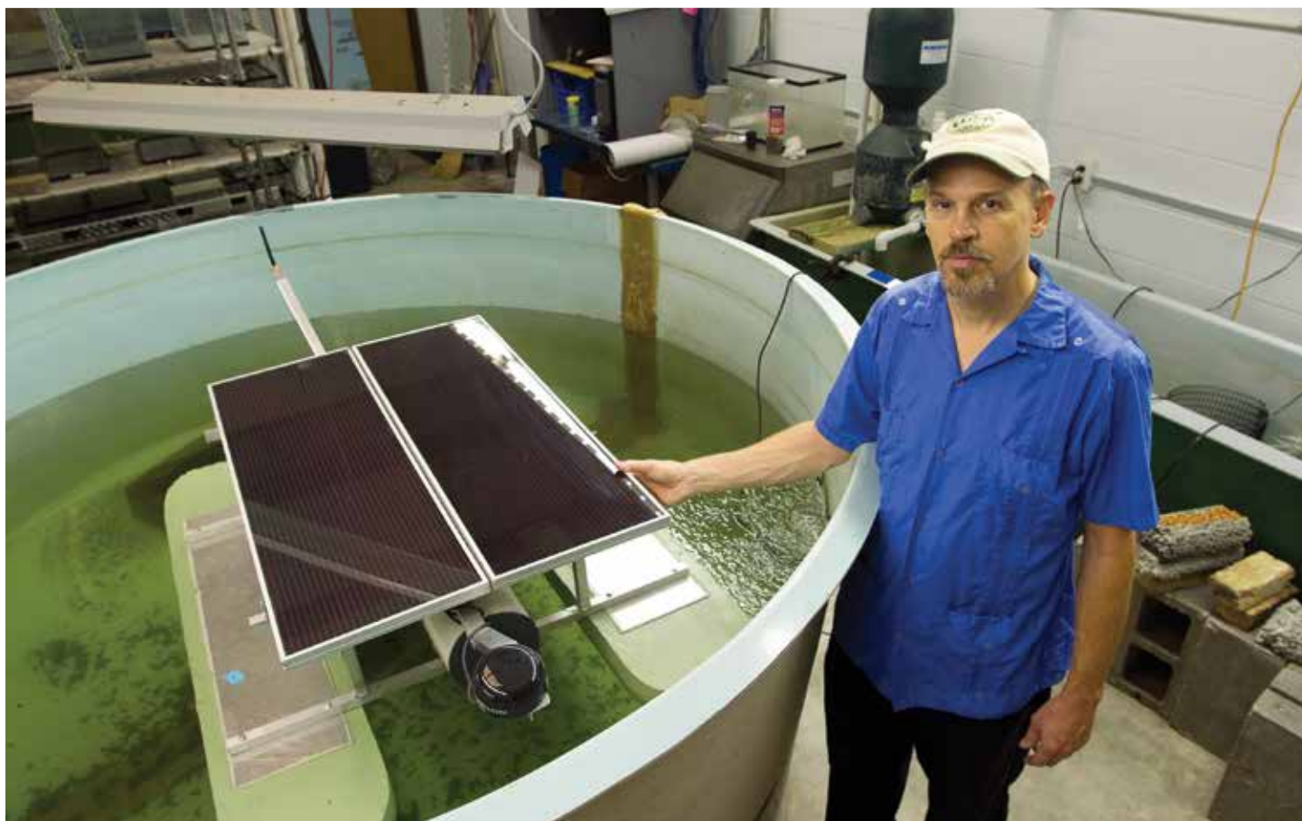
Steve Hall, researcher in the Department of Biological and Agricultural Engineering, with one of the robotic boats he has developed. The dual pontoon, dual paddlewheel automated boats are powered by the sun, microcontroller driven and may have a variety of sensors including GPS and water quality sensors. Photo by Olivia McClure
