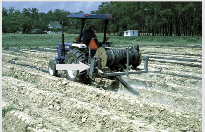
Figure 2. The vertical bar on the left of the spool is a swing arm that allows automatic adjustment of the spool speed. Note arrow.
