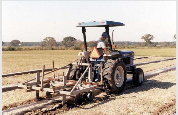
Figure 1. The primary purpose of this machine is to loosen and lift the plastic. It also slices the plastic which aids in soil removal.
