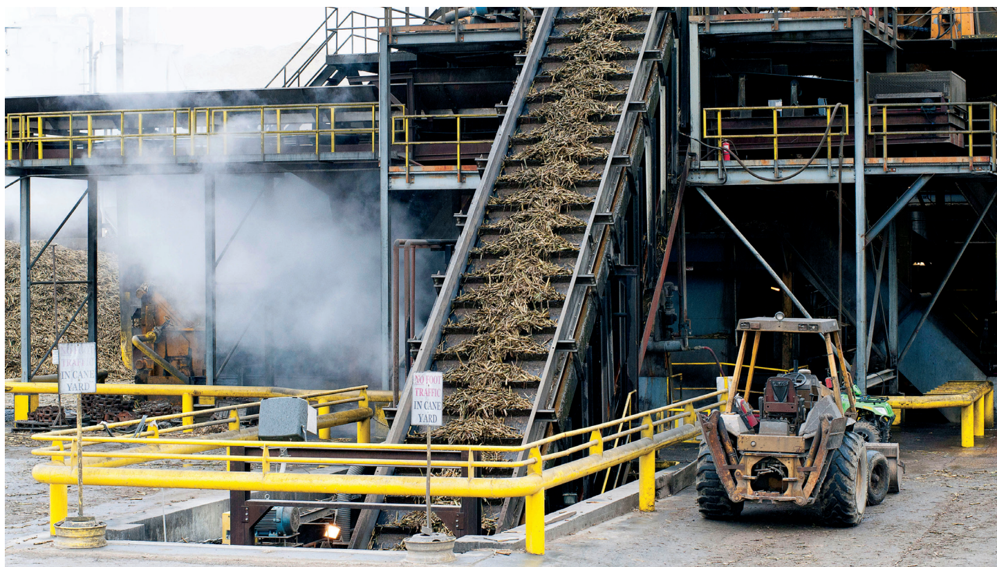
Alma Plantation in Lakeland, Louisiana, is one of 11 sugar factories in Louisiana. The sugarcane is brought to the mill where it is processed into sugar. Bagasse is the solid residue that remains after the extraction of juice from sugarcane. Photo by Olivia McClure
