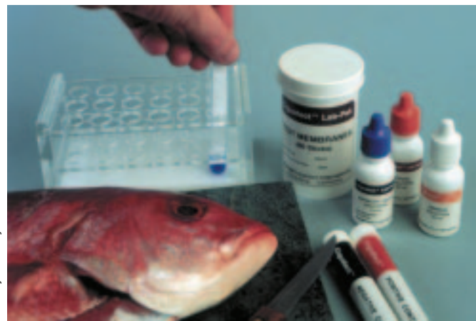
After a 10-minute incubation in immunobead solution, blue coloration of the membrane containing a sample denotes the presence of a specific marine biotoxin.
