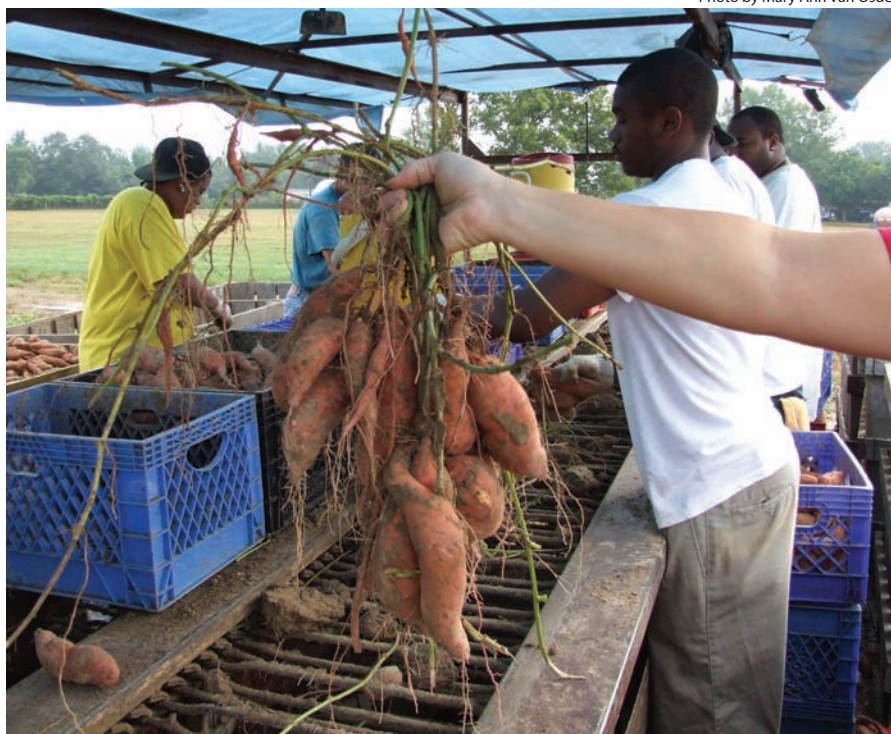
The sweet potato digger at the LSU AgCenter Sweet Potato Research Station at Chase, La., uses a blade that digs up the potatoes and walks the potatoes up a conveyor while shaking off the dirt to a place where workers then put the potatoes in bins.
